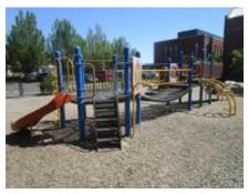
The play area has a garden area that was not located on an accessible route from the existing paved walkway and raised garden beds were located outside of accessible reach ranges.
